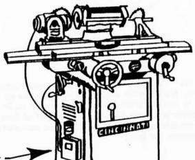
SOLID WHEBLS - Position nozzle downward, centered on the width of the wheel and about 1/16 th of the wheels circumference above the wheel/workpiece interface. Place the nozzle about 4 cm away from the wheel.
