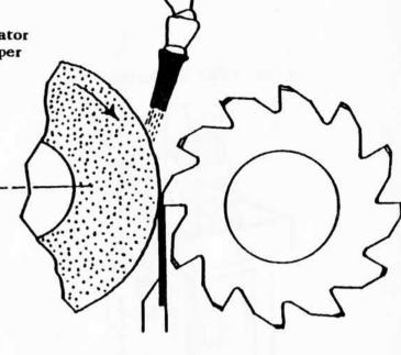
CUP WHEELS - Position nozzle downward at 12 o'clock position on the wheel, 2 cm away from the cup edge. Nozzle position is more critical on cup wheels because of the narrow wheel edge. Monitor nozzle position regularly to ensure proper lubrications with Accu-Lube.
